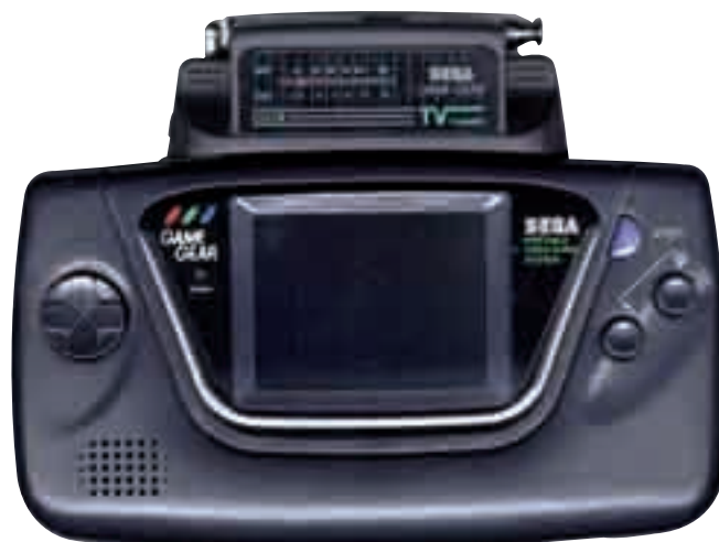
» The Game Gear Tuner is still highly collectable but won't work on later models or the Majesco-released machines.
